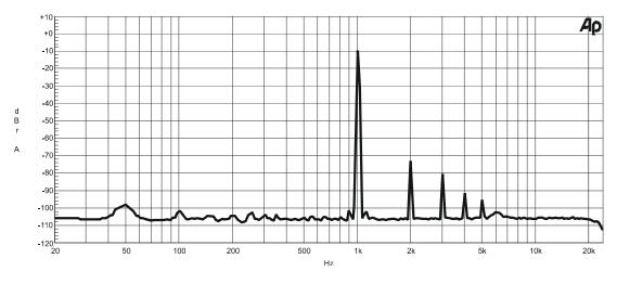
Noise spectrum at 1 kHz / 5 W into 4 ohms – there is no mains interference to be seen (50 Hz < 200  $\mu$ V, 100 Hz < 70  $\mu$ V). The k2, k3, k4 and k5 noise spectrum is extremely low and falls quickly.
