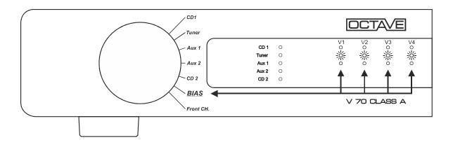
Five LEDs will now illuminate: The power LED and the 4 BIAS LEDs in the center of the display, one for each power tube. If the amplifier is still cold, the LEDs will initially illuminate "yellow".
