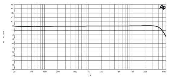
The frequency response curve clearly shows the low cut-off frequency of the V 70 class A; it is well below 20 Hz. The loss at 20 Hz is less than 0.2 dB
