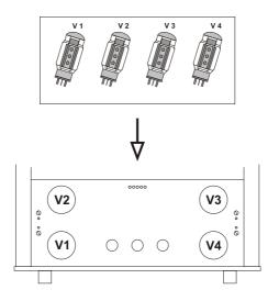
Insert the power tubes into their sockets as shown on the tube layout. Ensure that you correctly locate the anti-rotation lug on each of the tubes.
