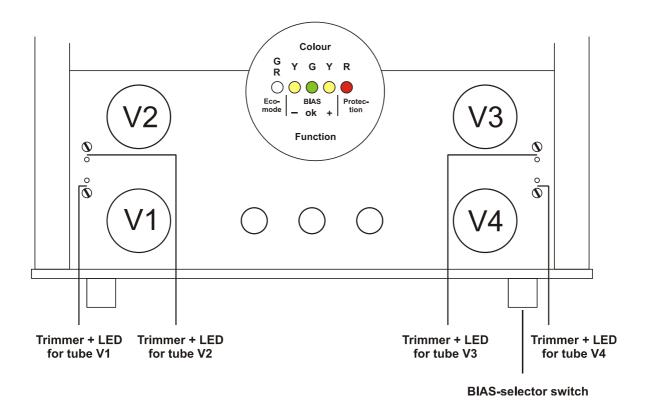
The BIAS measurement facility makes it easy for you to check and adjust the idle current of the output tubes. Getting the BIAS setting right for all four tubes is critical for both the sound of the power amplifier section and for the service life of the tubes. This feature guarantees consistent sound quality over the entire lifetime of the output tubes.
