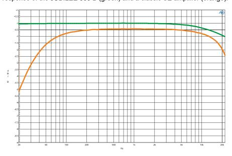
The frequency response of the JUBILEE 300 B is flat down to 20 Hz in the opposite to the low frequency roll off of a classic SE design.
