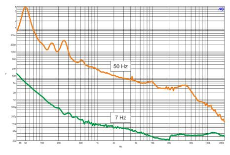
The distortions of the 7 Hz heating voltage are 200 times lower compared to the mains generated Heater voltage, thus mains distortions are ruled completely out.
