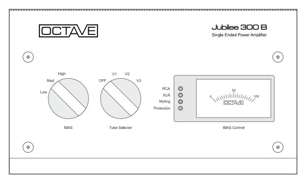
With the BIAS measuring device, the idle current of the end tubes is controlled. The correct BIAS adjustment of all three tubes is important for the sound characteristics of the power amplifier and the lifetime of the tubes. Therefore, a BIAS measuring device has been integrated in the JUBILEE 300 B, which makes it possible to control the BIAS without additional measuring devices.
